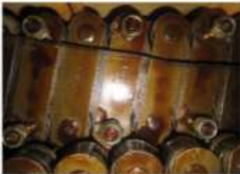
Solid Pin 4" 22.000 Lbf c/w Extended Pin Ev. 4 th Link 6" 42.000 Lbf c/w Extended Pin Ev. 4 th Link
