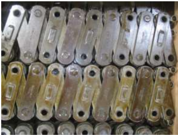
Solid Pin c/w Hollow Pin Every 4 th Link & 6 th Link
