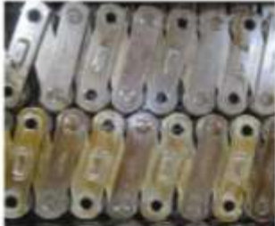
Solid Pin 4" 22.000 Lbf c/w Hollow Pin Ev. 4 th Link 6" 42.000 Lbf c/w Hollow Pin Ev. 4 th Link
